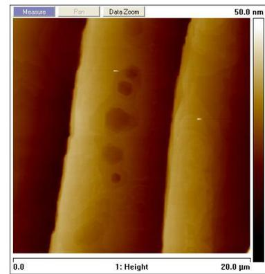
Figure 2: AFM image of graphene grown on Si face (annealed under H<sub>2</sub>, growth at high T°C for 30 min).
