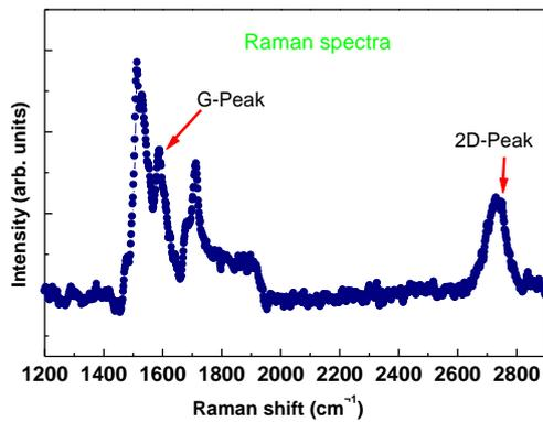
Figure 1: Raman spectra of graphene grown on Si face (annealed under H<sub>2</sub>, growth at high T°C for 30 min).
